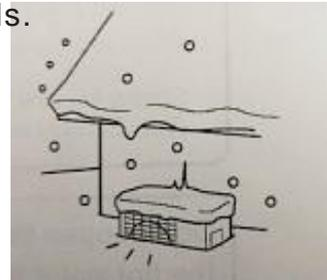
Snow building up around the heat pump unit and hot water storage tank unit could result in malfunction and failure.
